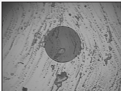
Fingerprint oil on endface
